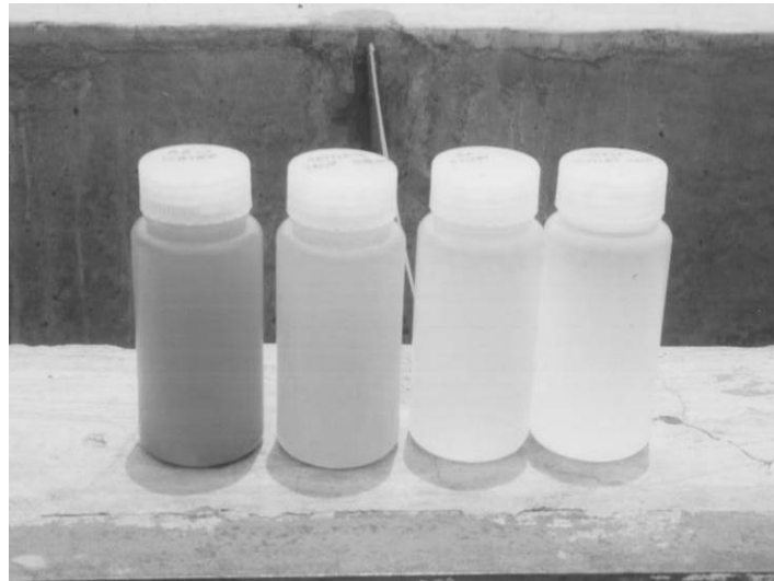
Figure 1: Improved water quality along MSF system (samples from: raw water, settling tank, pre-filter, slow sand filter – left to right).
